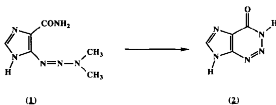
Figure 1 The structure of dacarbazine ( 1 ) and its main degradation product 2-azahypoxanthine ( 2 ).
